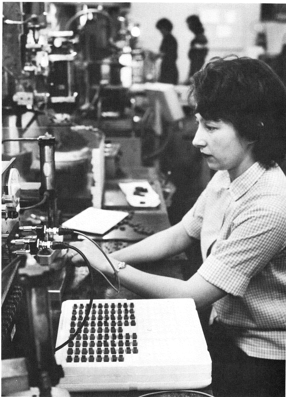
FIGURE 9 Magnetic measurement of ferrite cores. Here, pot core halves are assembled and measured for permeability. (Photo courtesy of Magnetics, Division of Spang & Co., Butler, PA.)
