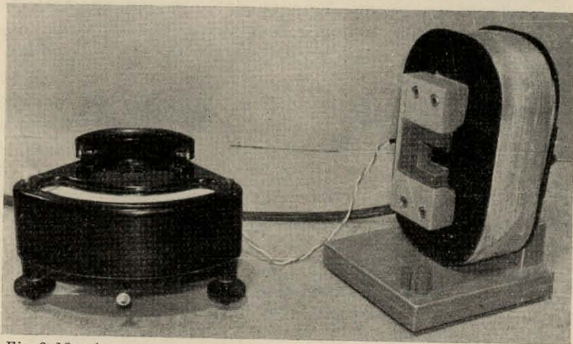
Fig. 3-16.—APPARATUS FOR TESTING MAGNETS UNDER CONTROLLED CONDITIONS OF DEMAGNETIZATION.
