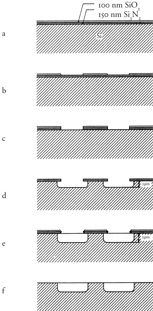
Figure 25. The LOCOS technique (from Philips Technical Review Vol. 31, p. 235).
