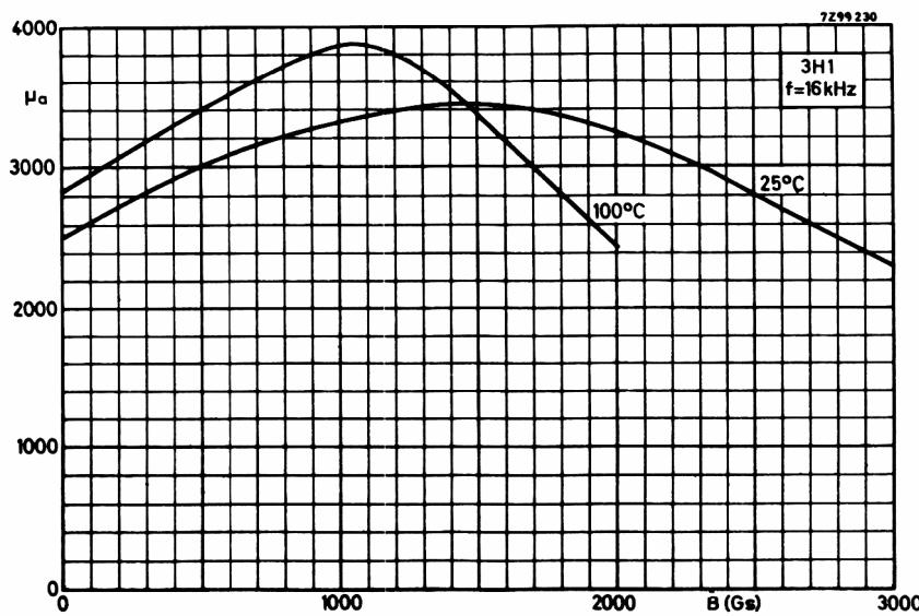
TYPICAL BH-CURVES (ballistically measured)
