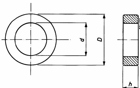
Ferroxcube toroids are used in small broadband transformers, pulse transformers, etc.
