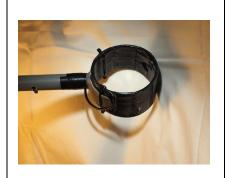
Coil form = plastic pipe. NO magnetic medium. N depends on pipe diameter, N should be equivalent to  $25 \times 25 \text{ cm}$  square. 1/16 sq. Meter. With 70 mm pipe N = 16.2.
